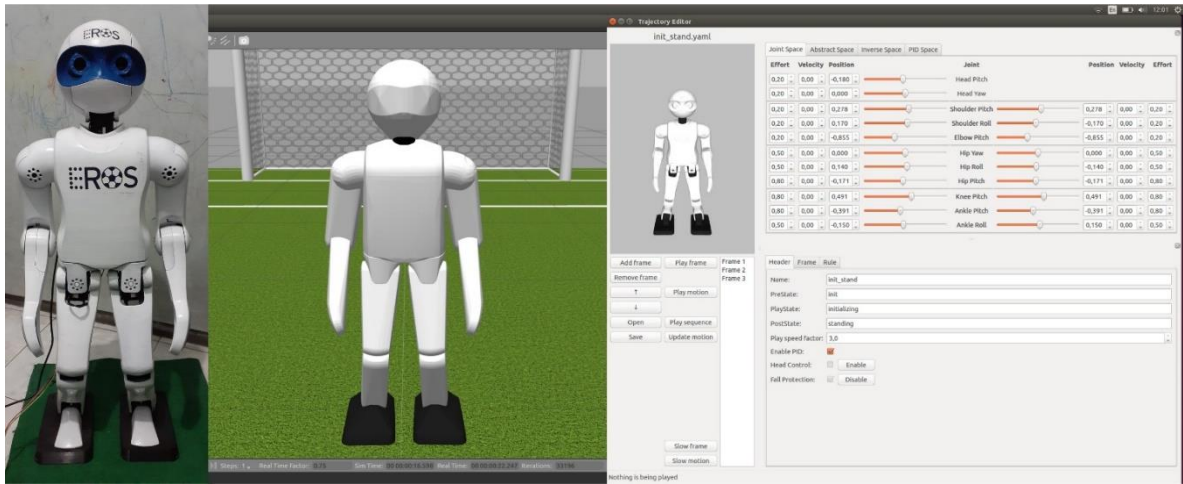
Figure 4. The appearance of the implementation of the whole gait generation. Starting from the rightmost picture that is making robot movements from the GUI (Graphical User Interface) that has been provided, switch to the image in the middle to simulate it on the ROS framework. The last step is the leftmost picture to practice directly on humanoid robots.
