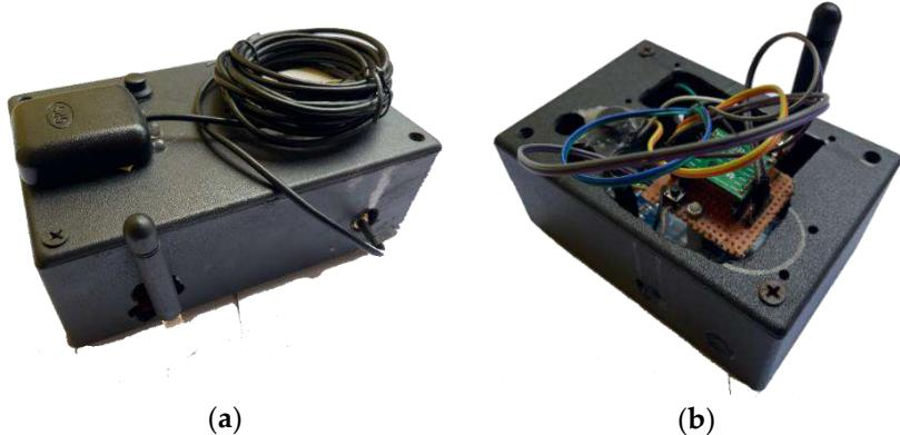
**Gambar 5.** Kotak perangkat keras: (a) *transmitter node*; (b) *receiver node*.
